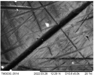
Fig. 4. Algae fibres, SEM image, contrast edited, magnification 5000x
