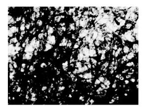
Fig. 7. Algae fibres, OM image by 720 nm, contrast edited, grayscale
