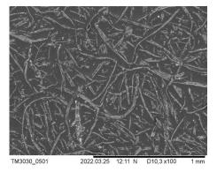
Fig. 2. Algae fibres on the paper surface SEM image, magnification 100x
