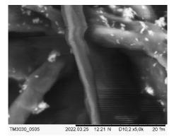
Fig. 3. Close-up of algae fibre on the paper surface, SEM image, magnification 5000x
